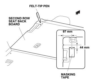
13. While wearing eye protection, drill the marked locations with a 3 mm drill bit, and then with a 5 mm drill bit. Drill through the hard board and the sheet metal. To prevent damage to the seat, wrap tape around the drill bit 25 mm from the tip as shown.
