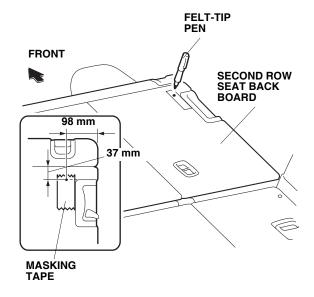
12. Using a felt-tip pen, measure and mark on the masking tape attached in step 10.
