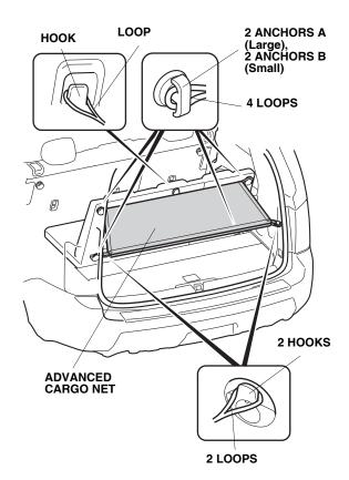
23. Attach two loops on the advanced cargo net to the two hooks.
