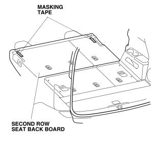
11. Using a felt-tip pen, measure and mark on the masking tape attached in step 10.
