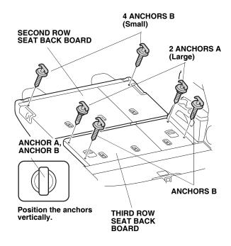
18. Install the four anchors B (Small) on the second and third row seat back boards into the holes made in steps 8 and 13.
