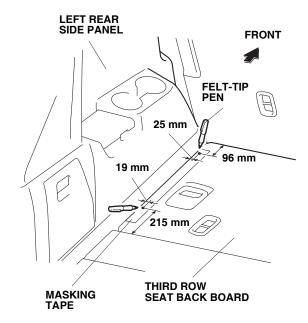
6. While wearing eye protection, drill the two forward marked locations with a 3 mm drill bit, and then with a 5 mm drill bit. Drill through the hard board and the sheet metal. To prevent damage to the seat, wrap tape around the drill bit 25 mm from the tip as shown.
