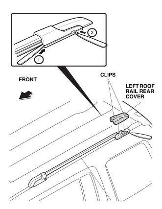
Slide the crossbars into the roof rails with the adjustment screws on the passenger's side of the vehicle. Align the marks on the crossbars with the marks on the roof rails as shown. Make sure the
