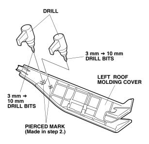
4. Enlarge the two holes with a 10 mm drill bit. Remove any burrs.
