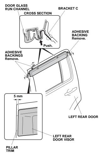
Remove the adhesive backings from the left rear door visor. 17. Using a rubber roller, apply pressure over the adhesive backings on the left rear door visor. Do not scratch the door visor with the rubber roller.
