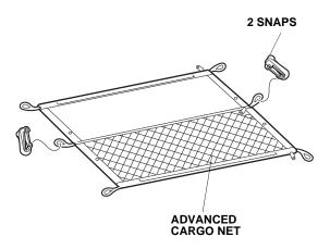
28. Attach four loops on the advanced cargo net to two hooks and two anchors B (Small) on the third row seat back board.
