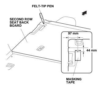
13. While wearing eye protection, drill the marked locations with a 3 mm drill bit, and then with a 5 mm drill bit. Drill through the hard board and the sheet metal. To prevent damage to the seat, wrap tape around the drill bit 25 mm from the tip as shown.
