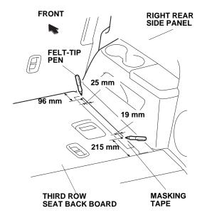
5. Using a felt-tip pen, measure and mark two locations on the masking tape.
