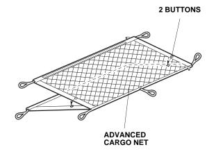
22. Attach five loops on the advanced cargo net to two anchors A (Large), two anchors B (Small) and the hook on the third row seat back board.
