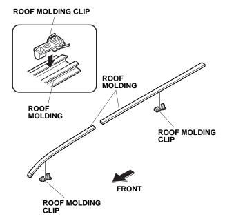
11. Reinstall the roof molding left cover.
