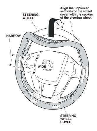
Pull back the edge of the steering wheel cover. Peel back the adhesive backings shown, and temporarily attach them to the front of the steering wheel cover with masking tape.
