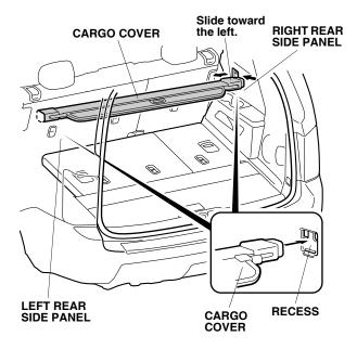
5. Pull out the cargo cover, and attach the right and left rods on the cargo cover to the right and left rear side panel.
