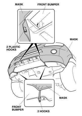
11. Attach the two hooks to the bottom edge of the front bumper as shown.
