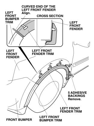
While applying light pressure against the left front fender trim, carefully remove the taped adhesive backings. 13. Hold the left front fender trim upward and bend the mounting tab around the left front fender. Using needle nose pliers over a shop towel, bend the mounting tab around the fender flange.
