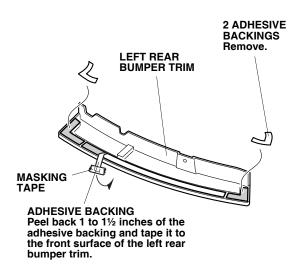
20. Align the edge of the left rear bumper trim with the curved end of the rear bumper as shown. Attach the left rear bumper trim to the rear bumper.
