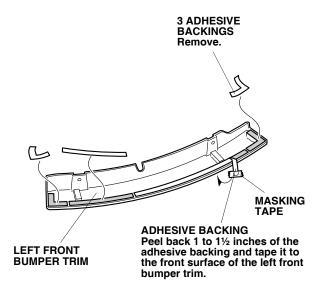
6. Align the edge of the left front bumper trim with the curved end of the front bumper as shown. Attach the left front bumper trim to the front bumper.
