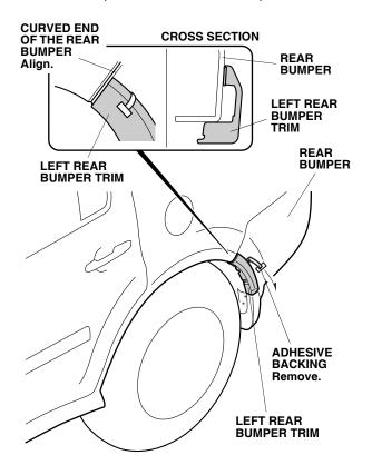
While applying light pressure against the left rear bumper trim, carefully remove the taped adhesive backing. 22. Install one screw (removed in step 16) to the left rear bumper trim.
