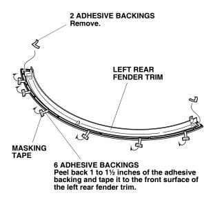
24. Align the edge of the left rear fender trim with the curved end of the left rear fender as shown. Attach the left rear fender trim to the left rear fender.
