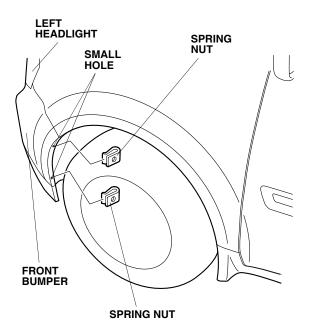
Check the position of the left front bumper trim and the left front fender trim to the front bumper and the left front fender. Remove the left front bumper trim and the left front fender trim.
