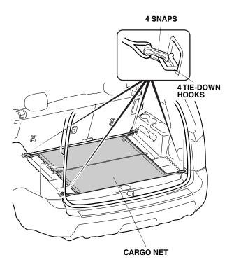
4. Attach four snaps on the cargo net to the four tie-down hooks in the cargo area.
