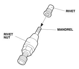
Insert the rivet nut into the hole in the vehicle frame and install the hex wrench on the rivet nut tool.
