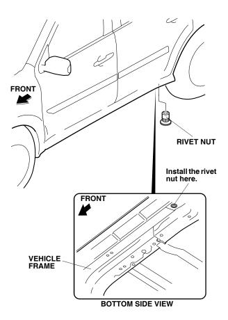
Screw the rivet nut onto the mandrel of the rivet nut tool as shown.
