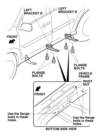
Position the left running board on the left bracket A and the two left brackets B. Install the left running board with six flange nuts. Do not tighten the flange nuts yet.
