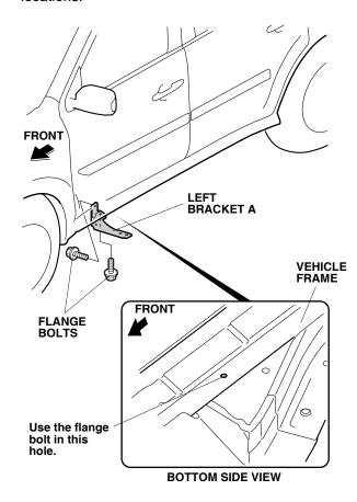
3. Install the two left brackets B on the vehicle frame using two flange bolts in each. Do not tighten the flange bolts yet. Make sure the flange bolts are installed in the correct locations.
