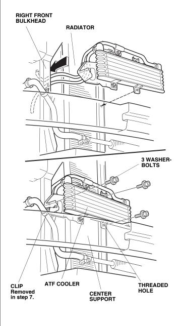
Install the clip on the power steering reservoir return hose (removed in step 7) into the clip hole in the ATF cooler.
