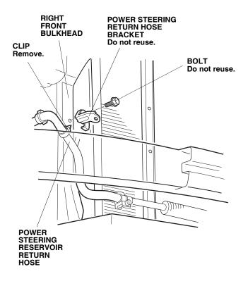
8. Remove the power steering return hose bracket (one bolt). The bolt and bracket will not be reused.
