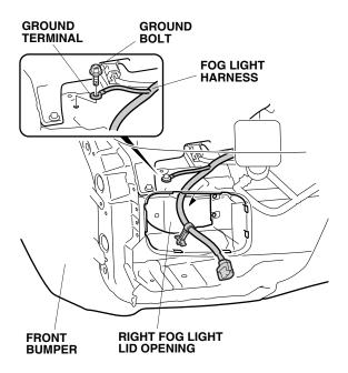
9. Pull the fog light harness 2-pin connector (shorter section of the harness) out of the right fog light lid opening.
