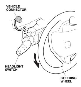
31. Remove the two self-tapping screws from the headlight switch. While pushing the retaining tab, slide the headlight switch, and remove it from the steering column. Do not pull on the lever when removing the case. Do not damage the tab hole in the steering column.
