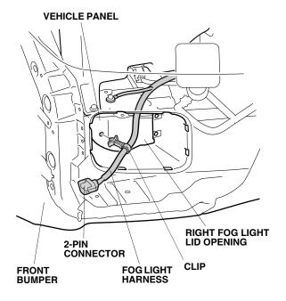
10. Secure the fog light harness clip to the vehicle panel.
