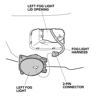
21. Insert the two hooks on the left fog light into the front bumper, and install the left fog light on the front bumper with two 5 x 16 mm washer-bolts.
