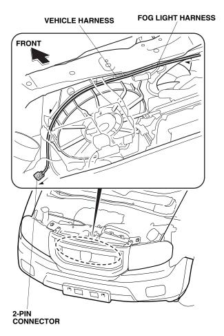
14. Route the fog light harness 2-pin connector to the underside of the vehicle.
