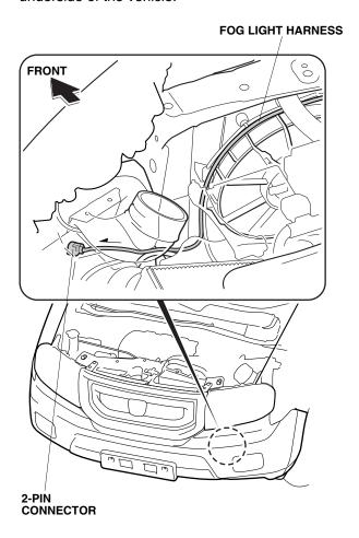
15. Pull the fog light harness 2-pin connector out of the left fog light lid opening.
