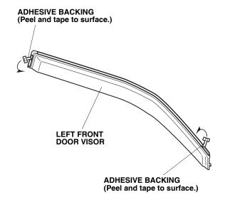
Using isopropyl alcohol on a shop towel, clean the door sash where the left front door visor will attach.
