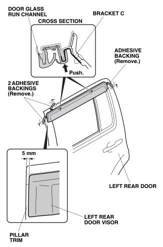
16. Remove the adhesive backings from the left rear door visor.
