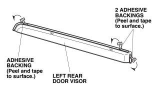
13. Using isopropyl alcohol on a shop towel, clean the door sash where the left rear door visor will attach.
