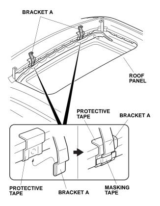
13. Align the holes in the moonroof visor with the holes in brackets A and B. Secure the moonroof visor to the brackets using the four screws and four nuts. Do not tighten the screws at this time.
