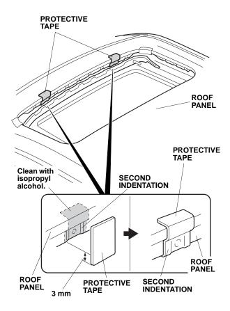
10. Locate the second indentation from the right front corner of the moonroof opening. Remove the adhesive backing from one protective tape. Starting from the bottom edge of the second indentation, wrap 6 mm of the protective tape around the lip of the roof panel opening. Wrap the remaining portion of protective tape up around the top of the roof panel. Install the protective tape to the second indent on the left side of the roof panel the same way.
