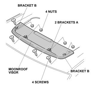
14. Adjust the position of the moonroof visor. Check that all of the brackets are firmly snug against the moonroof lip. Make sure the rubber molding on the moonroof visor is not twisted or rolled under the visor, and unfold if necessary.
