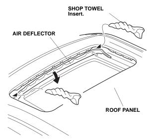
6. Roll up two shop towels and insert them between the roof panel and air deflector to lower the air deflector. Do not damage the air deflector.
