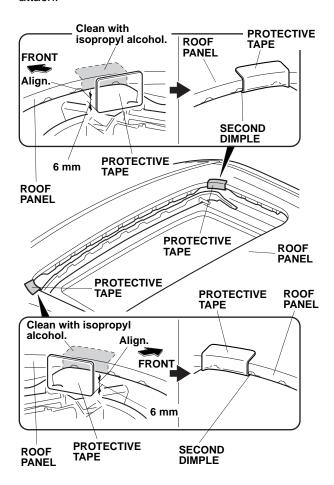
8. Locate the dimples at the right front corner of the moonroof opening. Remove the adhesive backing from one protective tape. Starting at the second dimple from the rear, wrap 6 mm of the protective tape around the bottom lip of the roof panel opening. Wrap the remaining portion of the protective tape up around the top of the roof panel. Install a protective tape to the left front corner of the moonroof opening the same way.
