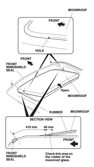
Using the measurements shown, check the rubber on the left and right side for a hole. If the rubber has a hole on either side, continue with step 3, otherwise, go to step 5. 3. Using a small phillips screwdriver, insert the sealer towards the rear side of the hole as shown.
