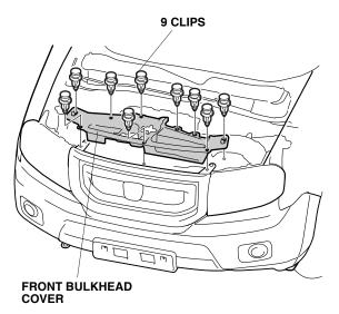
Remove the front bumper (nine clips, four bolts, and four self-tapping screws). Have an assistant help you when removing and installing the front bumper. If the vehicle is equipped with foglights or front corner sensors, unplug the connectors. Place the front bumper on a blanket after removal.
