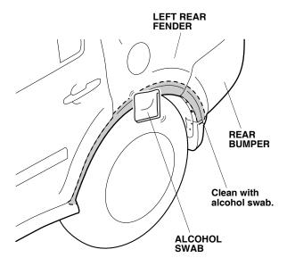
19. Peel back 1 to 1½ inches of the adhesive backing and tape it to the front surface of the left rear bumper trim. Remove the remaining adhesive backings from the left rear bumper trim.
