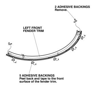
11. Align the edge of the left front fender trim with the curved end of the left front fender as shown.
