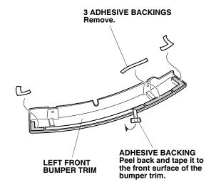
6. Align the edge of the left front bumper trim with the curved end of the front bumper as shown.
