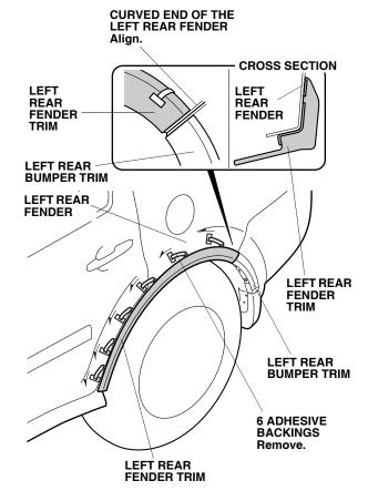
25. Attach the left rear fender trim to the left rear fender. While applying light pressure against the left rear fender trim, carefully remove the taped adhesive backings.
