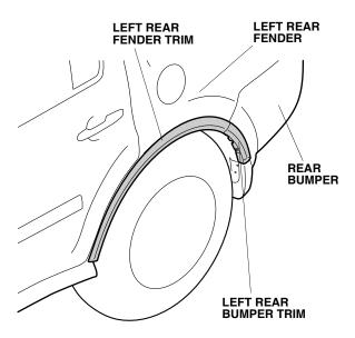
18. Using an alcohol swab, thoroughly clean the area where the left rear bumper trim and the left rear fender trim will be attached.
