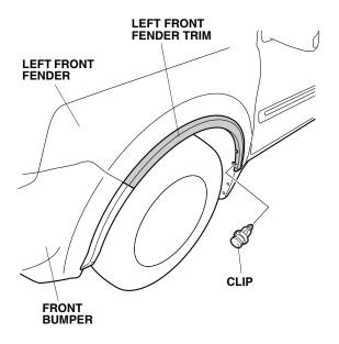
15. Using a rubber roller, apply pressure against the left front fender trim and left front bumper trim, and roll from one end to the other.
