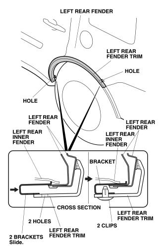
27. Install the two new clips at the left rear fender trim as shown.
