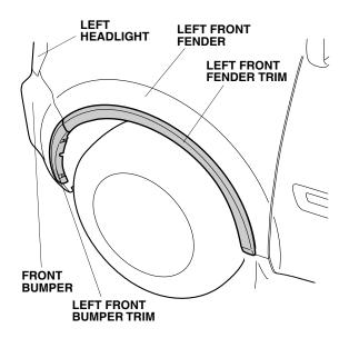
4. Using an alcohol swab, thoroughly clean the area where the left front bumper trim and the left front fender trim will be attached.
