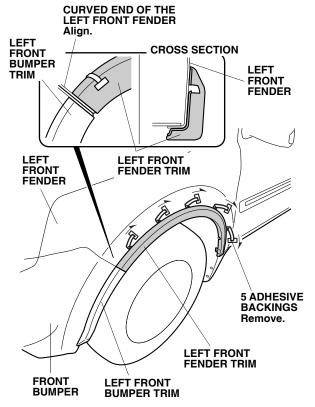
Attach the left front fender trim to the left front fender.
