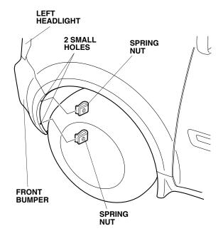
3. Position the left front bumper trim and the left front fender trim to the front bumper and the left front fender.
