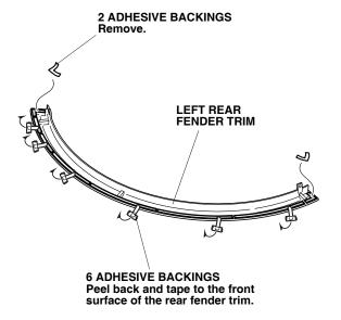
24. Align the edge of the left rear fender trim with the curved end of the left rear fender as shown.
