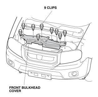
2. Remove the front bumper (nine clips, four bolts, and four self-tapping screws). Have an assistant help you when removing and installing the front bumper. If the vehicle is equipped with fog lights or front corner sensors, unplug the connectors.
