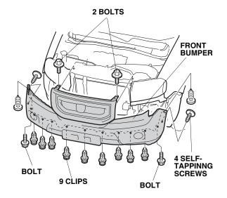
3. Remove the bumper grille from the front upper bumper and the front lower bumper (sixteen hooks).
