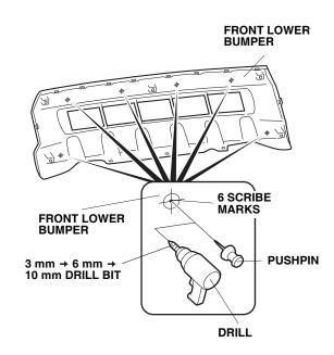
6. While wearing eye protection, first drill with a 3 mm drill bit, then drill with a 6 mm drill bit, and finish with a 10 mm drill bit. Remove all burrs.
