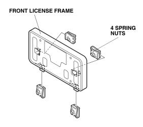
16. Install the front license frame to the front trim with four washer-bolts.
