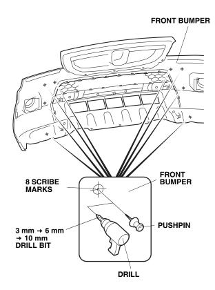
12. While wearing eye protection, drill with a 3 mm drill bit, then drill with a 6 mm drill bit, and finish with a 10 mm drill bit. Remove all burrs.
