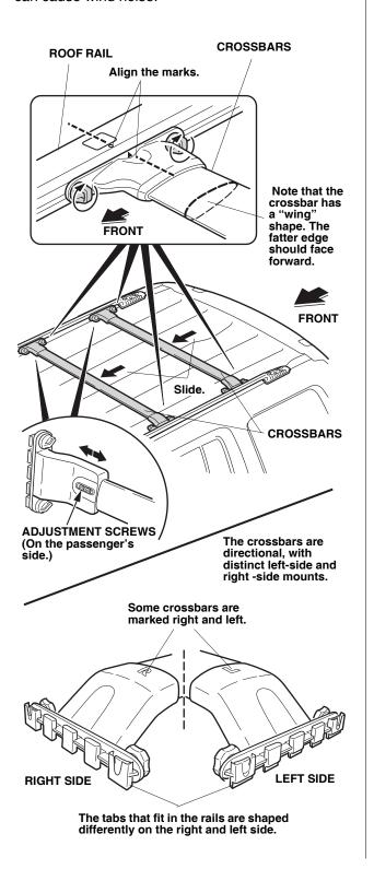
3. Tighten eight thumbwheel screws to secure the crossbars to the roof rails.
