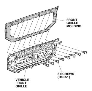
7. Remove the rubber molding from the vehicle front grille.
