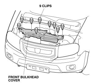
Remove the front bumper (nine clips, four bolts, and four self- tapping screws). Have an assistant help you when removing the front bumper. If the vehicle is equipped with foglights or front corner sensors, unplug the connectors. Place the front bumper on the blanket after removal.
