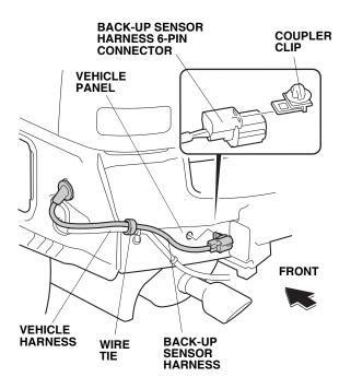
42. Secure the back-up sensor harness to the vehicle harness with one wire tie.
