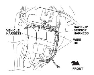
37. Remove the vehicle ground bolt from the vehicle ground terminal. Secure the back-up sensor harness ground terminal to the vehicle ground terminal with the vehicle ground bolt you just removed.
