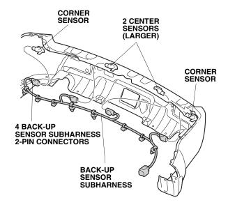
57. Attach three back-up sensor subharness clips (A) into three sensor clips.
