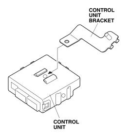
Secure the control unit bracket to the vehicle panel with the 6 mm flange nut.
