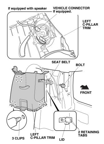
16. Using a small rubber mallet and a shop towel, gently tap the left C-pillar trim at the area marked "SIDE CURTAIN AIRBAG" to release the clip.
