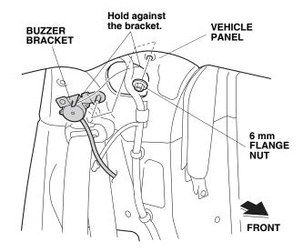
Secure the vehicle harness to the buzzer bracket with the offset wire tie as shown.
