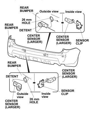
56. Plug the four back-up sensor subharness 2-pin connectors to the two corner sensors and two center sensors.
