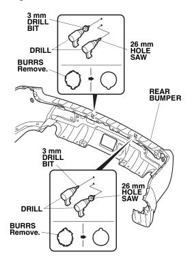
54. Install the two corner sensors on the rear bumper using one sensor clip for each sensor.
