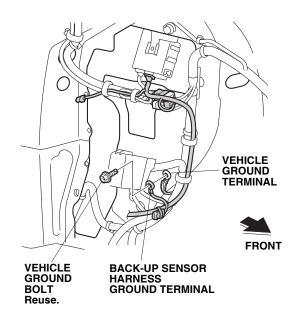
38. Route the back-up sensor harness on the rear side of the vehicle, and secure it to the vehicle harness with three wire ties.
