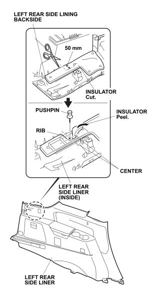
44. Using a pushpin, mark the left rear side liner in the center of the square as shown.
