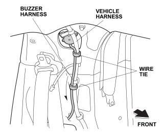
28. Secure the buzzer harness to the vehicle harness with three wire ties.
