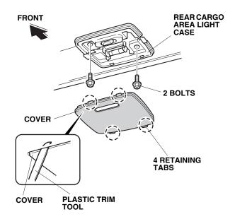
5. Remove the two bolts from the rear cargo area light case.
