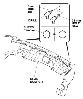
53. While wearing eye protection drill the right center mark at the upper pierced mark with a 3 mm drill bit. On the left center mark, drill the lower pierced mark with a 3 mm drill bit. Then drill the two center marks using a 26 mm hole saw. Remove all burrs.
