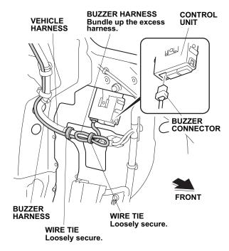
30. Loosely secure the buzzer harness to the vehicle harness with one wire tie.
