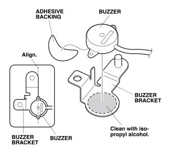
25. Using one 6 mm flange nut, secure the buzzer bracket to the vehicle panel in the position where the vehicle harness clip was removed in step 23.
