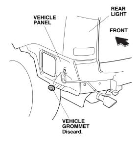
40. Route the back-up sensor harness through the vehicle grommet hole, and install the back-up sensor harness grommet onto the vehicle panel.
