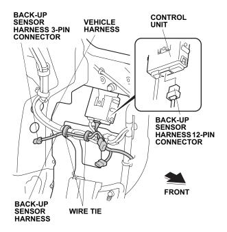
33. Route the back-up sensor harness 3-pin connector as shown and secure it to the vehicle harness with two wire ties loosely secured in step 29 and 30. 34. Unplug the vehicle 23-pin connector, and plug the back-up sensor harness 23-pin connector to the vehicle 23-pin connector as shown.
