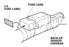
Plug the back-up sensor harness 12-pin connector to the control unit.
