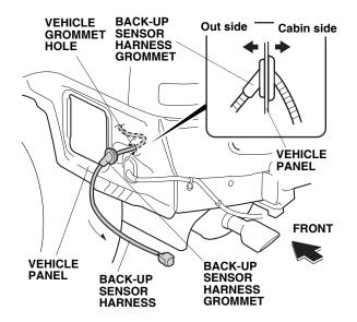
41. Slide the coupler clip onto the back-up sensor harness 6-pin connector, and secure it to the vehicle panel.
