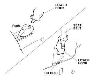
11. Remove the two seat belts from the left third row seat and remove the four bolts fastening the left third row seat to the floor. Remove the left third row seat.
