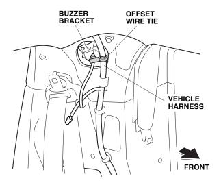
27. Route the buzzer harness along the vehicle harness, and secure it to the vehicle harness with two wire ties.
