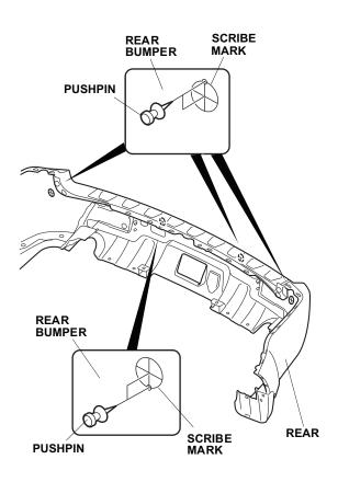
52. While wearing eye protection, drill at the upper out board pierced marks with a 3 mm bit. Drill the two outboard center marks using a 24 mm hole saw. Remove all burrs.
