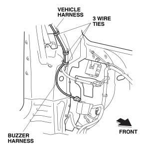
29. Plug the buzzer connector to the control unit. Bundle up the excess buzzer harness and loosely secure it to the vehicle harness with one wire tie.
