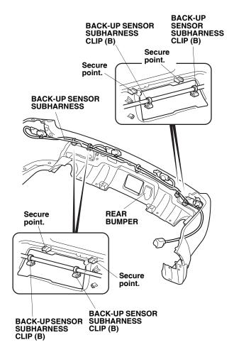
59. Using an isopropyl alcohol on a shop towel, clean the area where the harness tape will attach. Secure the back-up sensor subharness to the rear bumper with one harness tape.
