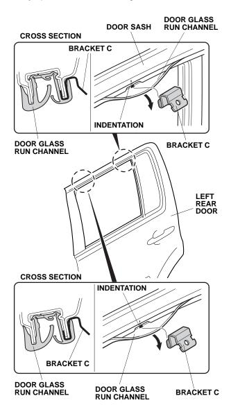
11. Peel the door glass run channel and install two brackets C to the left rear door as shown. Make sure that the brackets are installed in the correct position. Check that the brackets and the door glass run channel is installed on the door sash properly.
