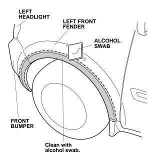
5. Peel back 1 to 1½ inches of the adhesive backing, and tape it to the front surface of the front bumper trim. Remove the remaining adhesive backings from the left front bumper trim.
