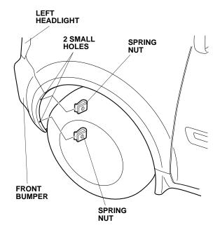
Position the left front bumper trim and the left front fender trim to the front bumper and the left front fender.
