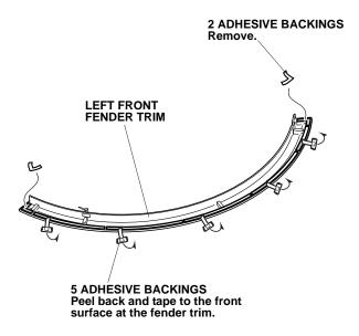
11. Align the edge of the left front fender trim with the curved end of the left front fender as shown.
