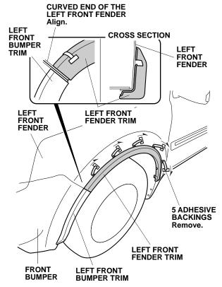
12. Attach the left front fender trim to the left front fender. While applying light pressure against the left front fender trim, and carefully remove the taped adhesive backings.
