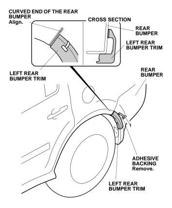
21. Attach the left rear bumper trim to the rear bumper. While applying light pressure on the left rear bumper trim, carefully remove the taped adhesive backing.
