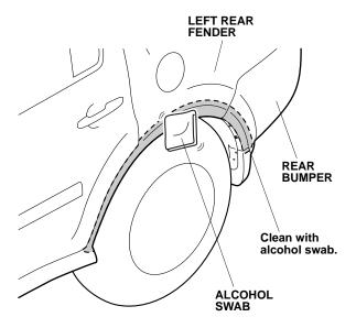
19. Peel back 1 to 1½ inches of the adhesive backing and tape them to the front surface of the left rear bumper trim. Remove the remaining adhesive backings from the left rear bumper trim.
