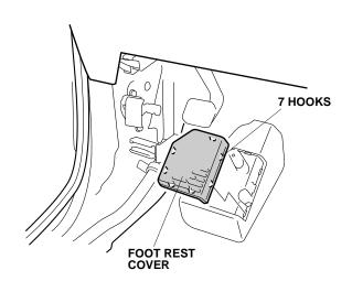
6. Remove the foot rest (two flange nuts).
