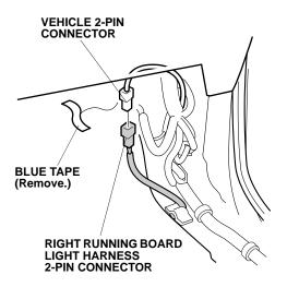
35. Plug the right running board light harness 2-pin connector into the vehicle 2-pin connector.
