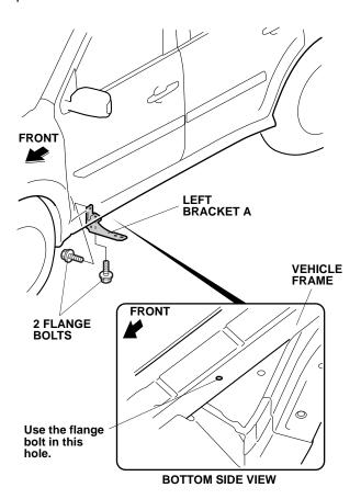
11. Position the two left brackets B at the respective installation positions of the vehicle frame. Install the two left brackets B on the vehicle frame with the two flange bolts for each. Do not tighten the flange bolts yet. Make sure the flange bolts are installed in the correct positions.
