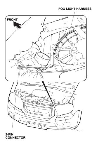
17. Pull the fog light harness 2-pin connector out of the left fog light lid opening.
