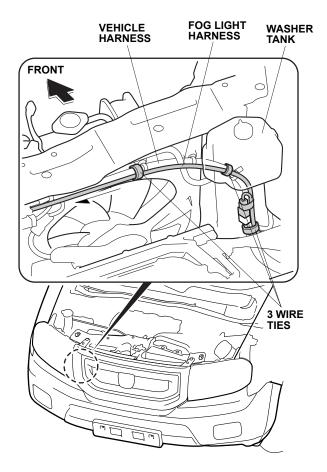
14. Secure the fog light harness to the vehicle harness with three wire ties.
