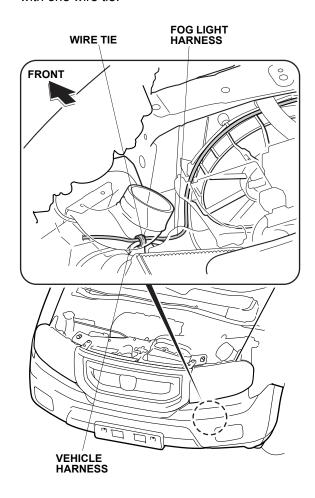
20. Secure the fog light harness to the vehicle harness with five wire ties.
