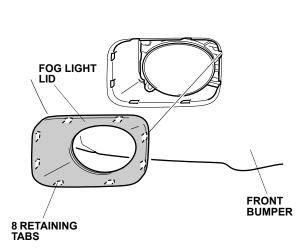
Remove the fog light (two washer-bolts, two hooks, and unplug the fog light 2-pin connector).
