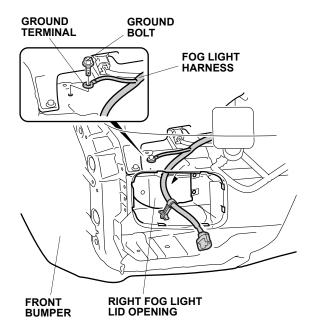
Pull the fog light harness 2-pin connector (shorter position of the harness) out of the right fog light lid opening.
