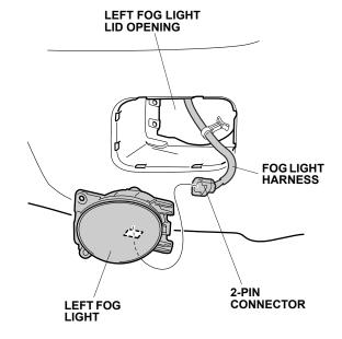
23. Insert the two hooks of the left fog light into the front bumper, and install the left fog light on the front bumper with two 5 x 16 mm washer-bolts.
