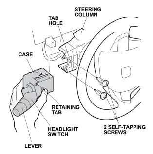
34. Install the new headlight switch on the steering column using the two self-tapping screws. Hold the case by hand, then install the new headlight switch to the steering column. Do not push the lever when installing the case. Push the case and set the retaining tab to the tab hole securely.
