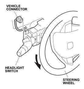
33. Remove the two self-tapping screws from the headlight switch. While pushing the retaining tab, slide the headlight switch, and remove it from the steering column. Do not pull out the lever when removing the case. Do not damage the tab hole of the steering column.
