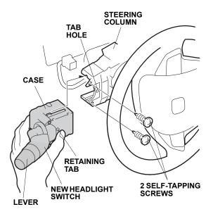
35. Plug the vehicle connector into the new headlight switch.
