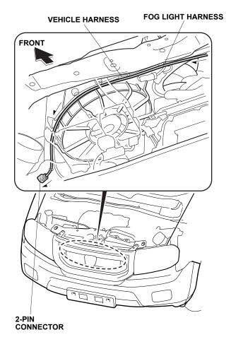
16. Route the fog light harness 2-pin connector (longer position of the harness) to the underside of the vehicle.
