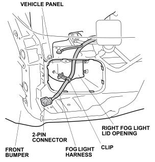
12. Secure the fog light harness clip to the vehicle panel.
