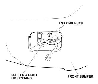
22. Plug the fog light harness 2-pin connector to the left fog light.
