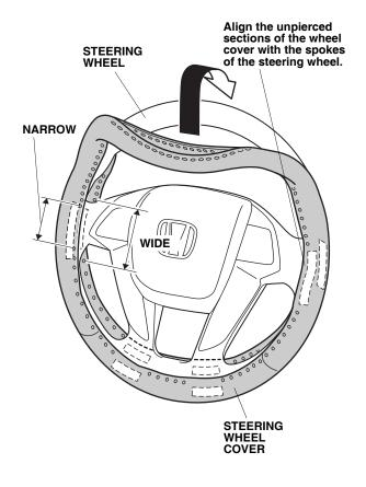
3. Turn over the steering wheel cover. Peel back the adhesive backings shown, and temporarily attach them to the front of the steering wheel cover with masking tape.
