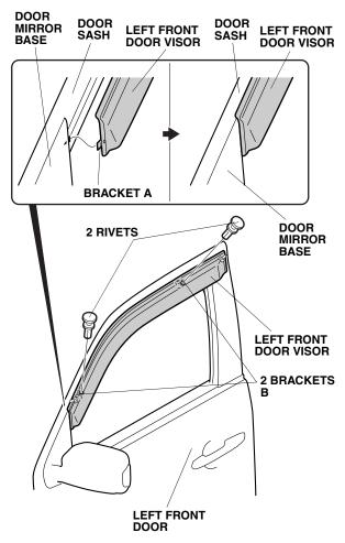
6. Align the holes on two brackets B to the holes on the left front door visor and secure it with two rivets.
