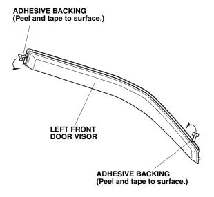
4. Using the isopropyl alcohol on a shop towel, clean the door sash where the left front door visor will attach.
