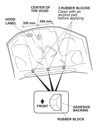
6. Remove the adhesive backings from three rubber blocks and hood label and attach them to the hood as shown.
