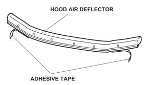
13. Align the holes on the hood air deflector with the brackets A, B, and C. Install the hood air deflector with two screws, two collars, and four clips. Tighten the screws securely. Remove the adhesive backings.
