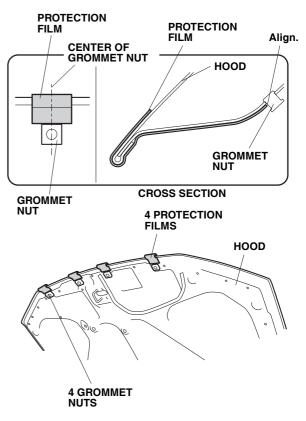
3. Remove the adhesive backings from the protection films and attach four protection films around the front of the hood as shown.
