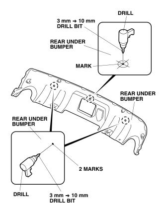
While wearing eye protection, drill four lower marks on the rear under bumper. First drill with a 3 mm drill bit and finish with a 10 mm drill bit, and remove all burrs.
