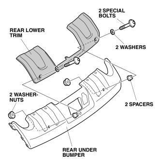
8. Secure the rear lower trim to the rear under bumper with four bolts.
