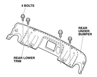
9. Reinstall the rear under bumper to the rear upper bumper.
