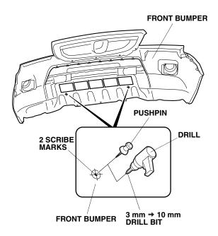
4. While wearing eye protection, first drill with a 3 mm drill bit and finish with a 10 mm drill bit, and remove all burrs.
