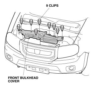
2. Remove the front bumper (nine clips, four bolts, and four self-tapping screws). Have an assistant help you when removing and installing the front bumper. If the vehicle is equipped with the foglight or the front corner sensors, unplug the connectors. Place the front bumper on a blanket after removal.
