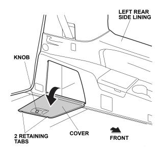
4. Pull the knob, and remove the cover from the left rear side lining (six retaining clips and two hooks).
