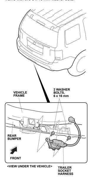
12. Release the vehicle 10-pin connector from the connector clip, and remove the dummy connector from the vehicle 10-pin connector.
