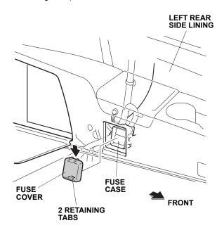
18. Plug the two 7.5A fuses and one 20A fuse to the fuse case.
