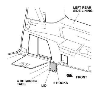
17. Remove the fuse cover from the fuse case (two retaining tabs).
