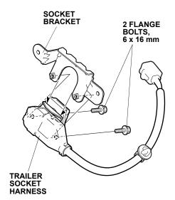
11. Secure the trailer socket harness to the vehicle frame with two 6 x 16 mm washer bolts.
