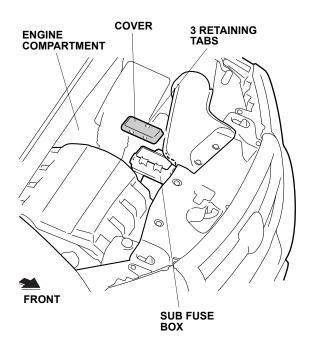
21. In the engine compartment, remove the cover from the sub fuse box (three retaining tabs).
