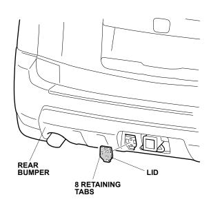
9. Using a utility knife, cut out the rear bumper from the lid opening as shown.
