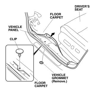
18. Remove the vehicle grommet of the vehicle panel.
