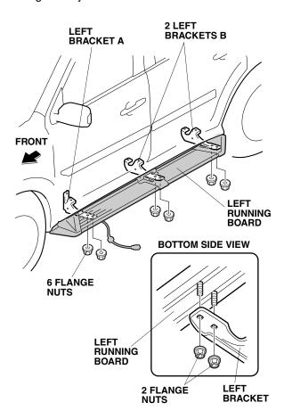
13. Align the front left running board with the left front door edge as shown.
