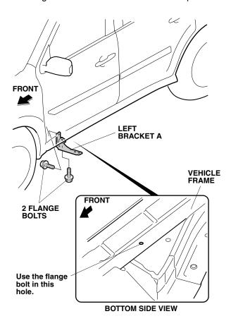
11. Position the two left brackets B at the respective installation positions of the vehicle frame. Install the two left brackets B on the vehicle frame with the two flange bolts for each. Do not tighten the flange bolts yet. Make sure the flange bolts are installed in the correct positions.
