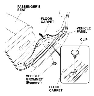
28. Remove the vehicle grommet from the vehicle panel.
