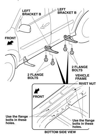
Position the left side step on the left bracket A and two left brackets B. Install the left side step with the six flange bolts. Torque the flange bolts to 27 N·m (19 lbf·ft).
