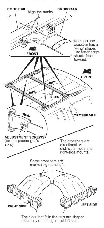
3. Tighten eight thumbwheel screws to secure the crossbars to the roof rails.
