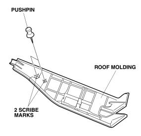
3. While wearing eye protection drill two holes on the roof molding at the holes made in step 2 with a 3 mm drill bit.
