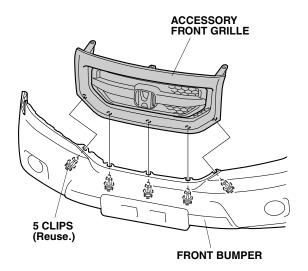
12. Reinstall the front bumper to the vehicle with nine clips, four self-tapping screws and four bolts. Have an assistant help you when installing the front bumper. If the vehicle is equipped with the foglights or the front corner sensors, plug the connectors.
