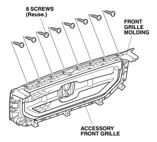
11. Install the accessory front grille to the front bumper with five clips removed in step 3.
