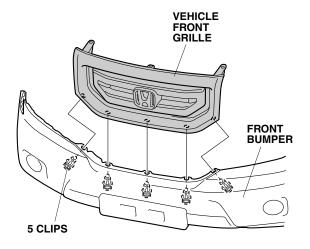
Separating the *vehicle* front grille from the front grille molding
