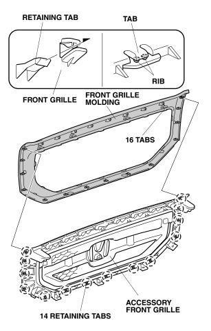
10. Secure the front grille molding to the accessory front grille with eight screws removed in step 6.
