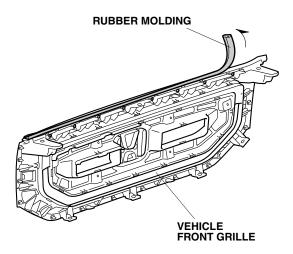
8. Install the rubber molding removed in step 7,to the accessory front grille
