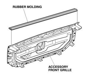
Installing the *front* grille molding to the accessory front grille
