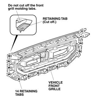
5. Cut off sixteen areas on the vehicle front grille as shown. Do not damage the front grille molding tabs when cutting the vehicle front grille.
