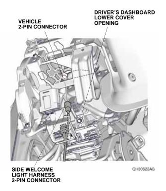
31. Secure the side welcome light harness to the vehicle harness with two wire ties.
