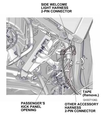
50. Bundle up the excess side welcome light harness, and secure it and 2-pin connectors to the vehicle harness with two wire ties as shown.
