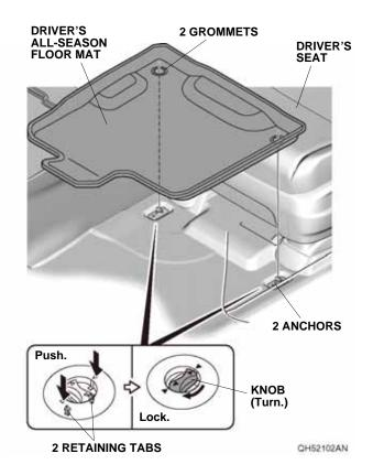
3. Place the grommets in the passenger's all-season floor mat over the anchors. Push the grommets into the anchors to secure the retaining tabs, then turn the knobs 90° to secure the passenger's all-season floor mat.
