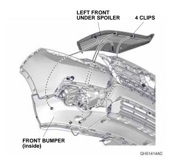
13. Secure the left front under spoiler to the front bumper with the four clips.
