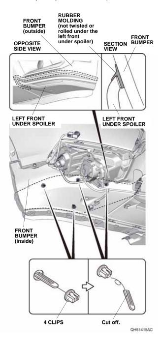
14. Secure the left front under spoiler to the front bumper with one washer and one 4 x 16 mm self-tapping screw.
