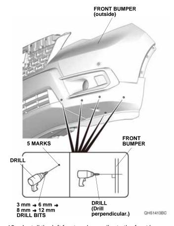
12. Install the left front under spoiler to the front bumper.
