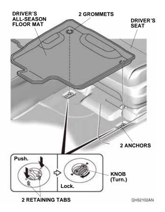
Place the grommets in the passenger's all-season floor mat over the anchors. Push the grommets into the anchors to secure the retaining tabs, then turn the knobs 90° to secure the passenger's all-season floor mat.
