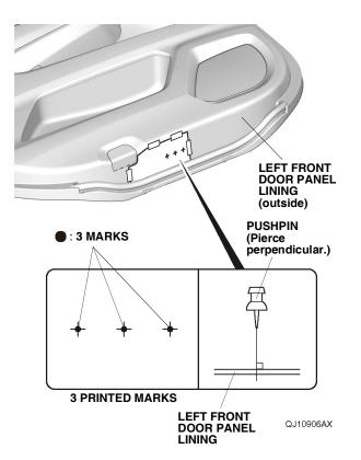
9. While wearing eye protection, drill the three pierced marks with a 3 mm drill bit from the outside of the left front door panel lining.
