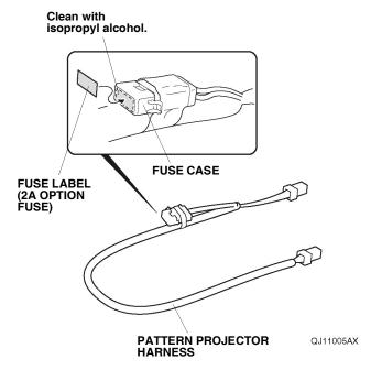
15. Plug the two pattern projector harness 2-pin connectors into the vehicle 2-pin connector and left light 2-pin connector.
