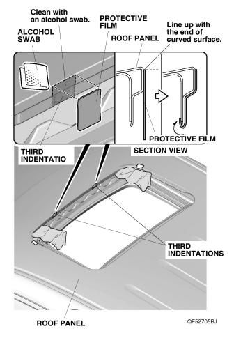
7. Remove the adhesive backing from the two protective films and attach one to the roof panel at each third indentation.
