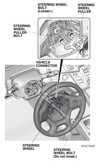
9. Using a steering wheel puller, release the steering wheel.
