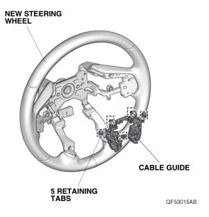
30. Install the new cable reel cord to the cable guide with the washer-screw removed in step 27. Plug the new cable reel cord 4-pin connector into the new steering wheel 4-pin connector, and secure the new cable reel cord to the cable guide.
