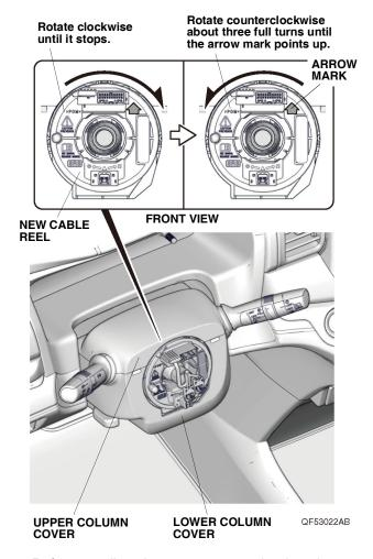
37. Before installing the new steering wheel, make sure the front wheels are still pointing straight-ahead. To confirm the cable reel is lined up properly, rotate the new cable reel clockwise until it stops, then rotate it counterclockwise about three full turns. The arrow mark on the new cable reel label must point straight
