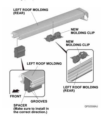
Install the left roof moldings back onto the roof of the vehicle as shown.
