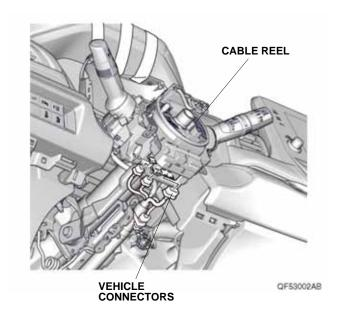
17. To prevent the cable reel from turning, apply masking tape to the cable reel. Remove the cable reel.
