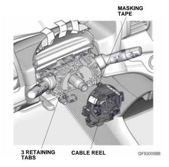
18. Remove the masking tape. Remove the steering angle sensor.
