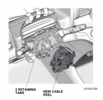
22. Plug the vehicle connectors into the new cable reel, and remove the locking pin.
