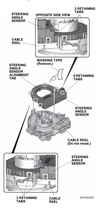
Install the steering angle sensor to the new cable reel.
