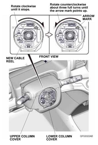
37. Before installing the new steering wheel, make sure the front wheels are still pointing straight-ahead. To confirm the cable reel is lined up properly, rotate the new cable reel clockwise until it stops, then rotate it counterclockwise about three full turns. The arrow mark on the new cable reel label must point straight up.
