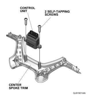
33. Plug the new cable reel cord 14-pin connector into the control unit, and install the center spoke trim to the new steering wheel with the two self-tapping screws removed in step 25.
