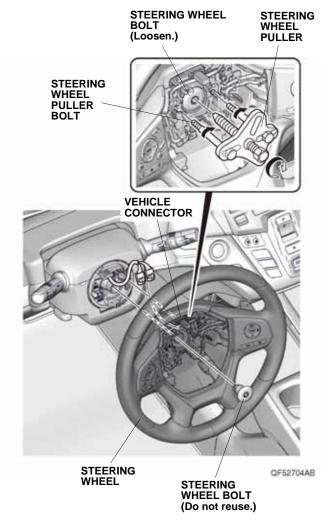
9. Using a steering wheel puller, release the steering wheel.
