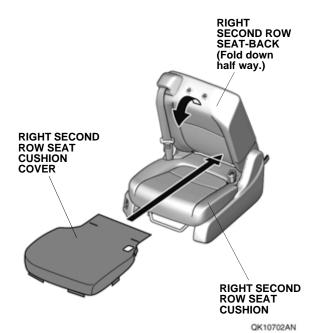
4. Secure the right second row seat cushion cover to the right second row seat cushion with four tabs and two fasteners.
