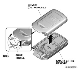
Install the new cover to the smart entry remote. If the vehicle is equipped with a cover marked DRIVER 1, install the new DRIVER 1 cover on that remote. NOTE: Make sure the new cover is completely snapped and properly sealed.
