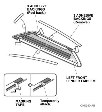
5. Line up the left front fender emblem with the template A, and attach it to the left front fender as shown.
