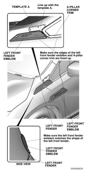
6. Make sure the edges of the left front fender emblem and A-pillar corner trim are lined up, and the left front fender emblem matches the shape of the left front fender.
