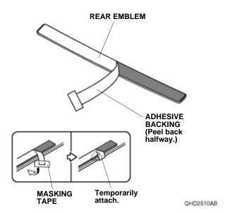
13. Line up the rear emblem with the template B, and attach it to the tailgate as shown.
