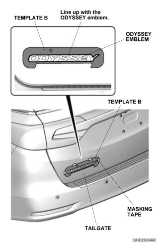
11. Using the alcohol wipe, thoroughly clean the tailgate where the rear emblem will attach.
