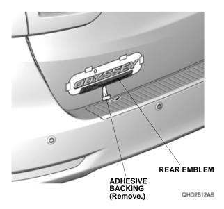
Using a rubber roller, apply firm pressure against the rear emblem and roll from one end to the other. Remove the template B.
