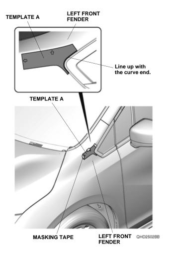
Line up the left front fender emblem with the template A. Make sure the edges of the left front fender emblem and A-pillar corner trim are lined up, and the left front fender emblem matches the shape of the left front fender.
