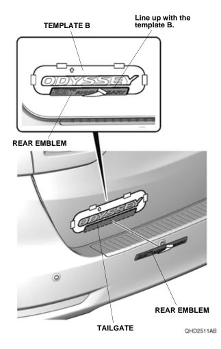
14. While applying light pressure against the rear emblem, carefully remove the taped adhesive backing.
